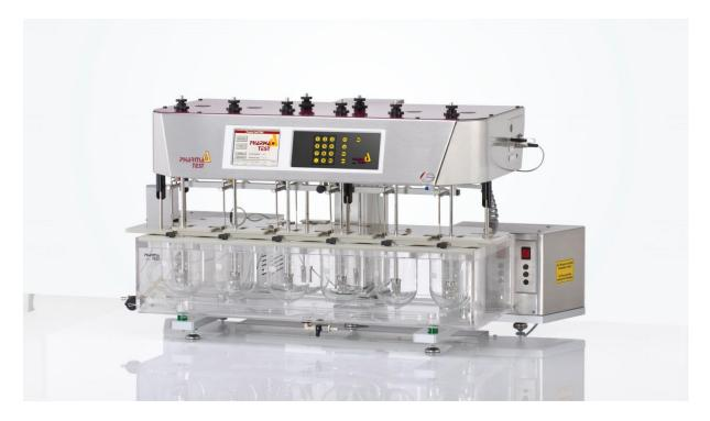
The PTWS 620 is a 6 + 2 position, single drive tablet dissolution testing instrument for solid dosage forms as described in USP chapter <711/724> and EP section<2.9.3/4> as well as the DAB/BP and Japanese Pharmacopeia section <15>. The USP monograph <1092/2.4.2> lists visual observation of the dissolution behavior as essential for identifying variables in the formulation or manufacturing process. The six vessels in the front row of PTWS 620 offer optimal visibility of the samples.
